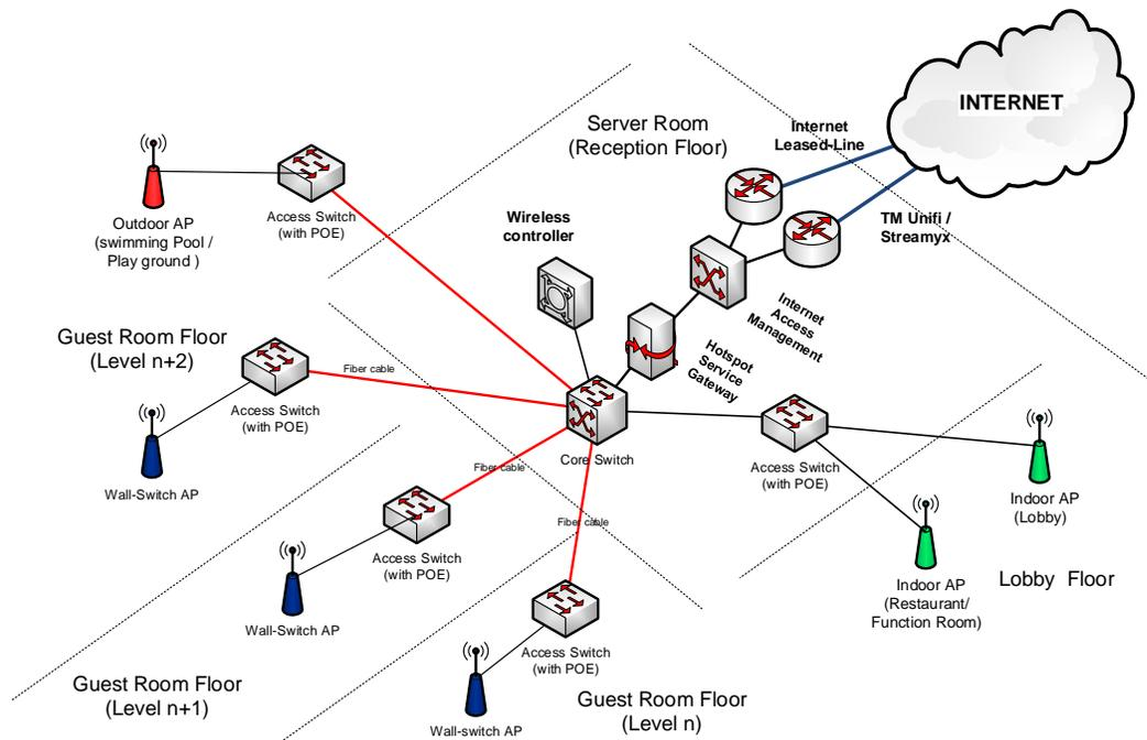
Figure 4: High-Speed Internet Access (HSIA) Architecture
