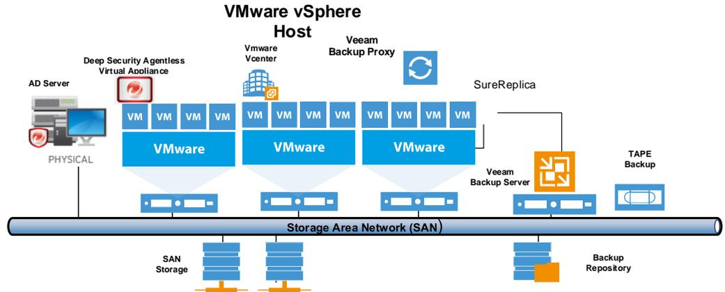
Figure 3: Typical Server Virtualization Architecture
