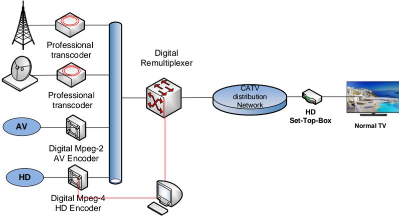
When the DTV broadcasts the digital video signals, it maintains higher picture quality than analogue signals because the picture information is already digitized. The digitized signal is free from snowing picture, ghosting, noise or interference and saving transmission bandwidth with MPEG-2 video compression technique.
