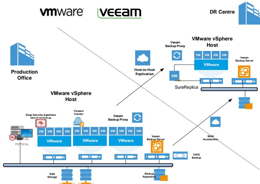
Figure 4: Data Backup and Replication Architecture
